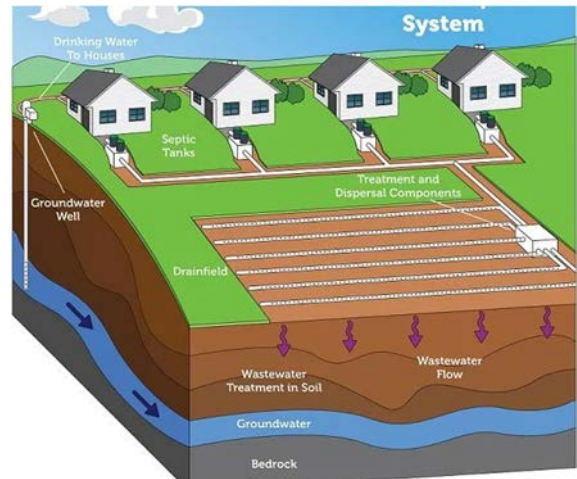
Cluster septic systems consolidate treatment and disposal in an efficient centralized system. However, sufficient land area, soil conditions, and funding are required. (Source: US Environmental Protection Agency)
